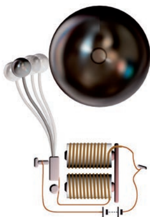
Fig. 14.20 Circuit of an electric bell
