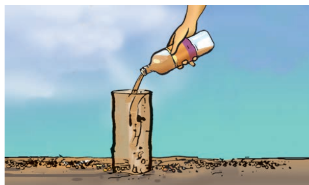
Fig. 9.5 Measuring rate of percolation
