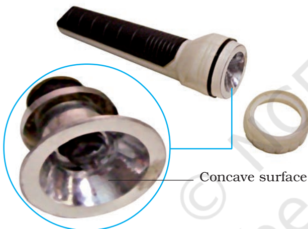
Fig. 15.18 Reflector of a torch
