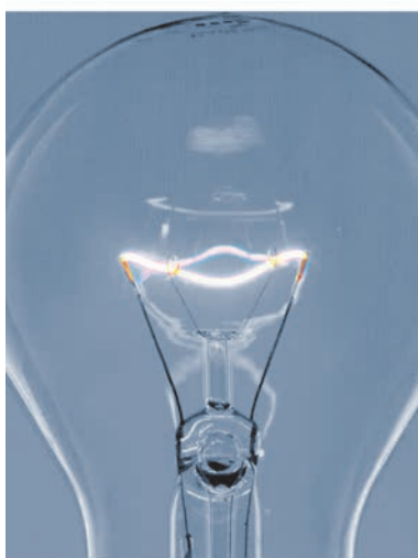
Fig. 14.12 Glowing filament of an electric bulb (incandescent)
